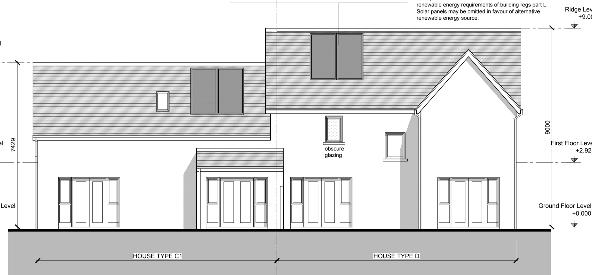
REAR ELEVATION House Type C1 - Semi-Detached
